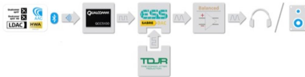
The digital-to-analogue conversion is performed by the ESS Sabre Hyperstream DAC chip. The signal from SOC has a huge amount of jitter. The ESS Sabre chip has Domain Jitter Elimination and a discrete oscillator so this eliminates jitter for the conversion to analogue. Once the conversion is complete, it is then sent to the amplifier.
