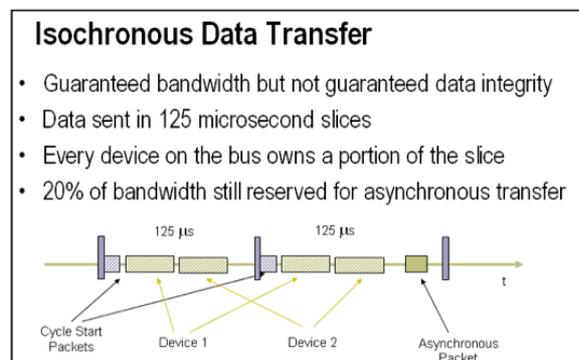
Isochronous mode is used for media streaming because it guarantees bandwidth on the USB bus by scheduling one transfer per available frame. By comparison Bulk or Burst transfers make use of 'leftover' bandwidth and may be 'choked off' if higher priority isochronous data transfers saturate the USB Bus.
