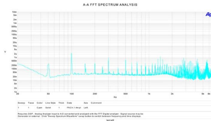
**Ap** The FFT noisefloor is around three times that of the AP2 itself at around 30nV (0.0000003V). We can also see that, as it should be for a power-supply, 100Hz is the highest peak at 3uV (0.000003V). And other high peaks are at multiples of 100Hz (not 50Hz...).
