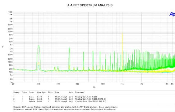
**Ap** As the **green** trace above shows, we sure do, not just 50Hz but we get an extended spray of harmonics all the way to the frequency limit.
