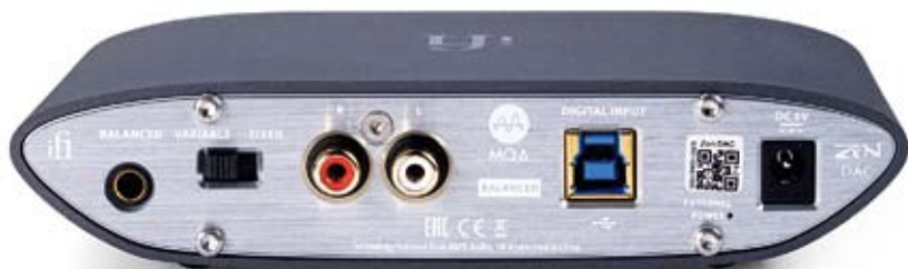
ABOVE: USB-hub powered (or via an external 5V PSU), the ZEN includes a USB-B digital in with both fixed/variable single-ended (RCA) and balanced (2.5mm) outs
