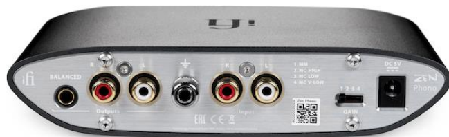
Around the back reside stereo RCA inputs/outputs, a 4.4mm Pentaconn balanced output, a grounding terminal and the gain selector switch
