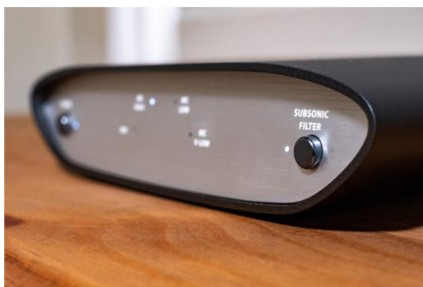
The ZEN Phono's front panel sports a 'subsonic filter' button, as well as LEDs to indicate the selected gain setting
