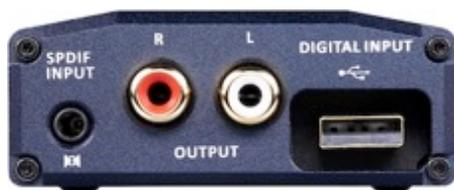
Between the digital inputs reside a pair of RCA analogue outputs – the micro iDSD
