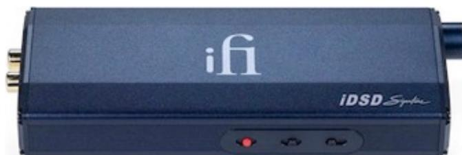
Hi-res audio support is state-of-the-art, handling PCM data to 32-bit/768kHz, all levels of DSD up to DSD512, and single- and double-speed DXD. MQA – the hi-res streaming codec, as used by Tidal's 'Masters' tier – is also supported. Thanks to the Burr-Brown chip's True Native design, PCM and DSD take separate pathways – this enables DSD, as well as PCM, to remain 'bit-perfect' in its native form right through to analogue conversion. This is often not the case with DAC devices from other brands.
