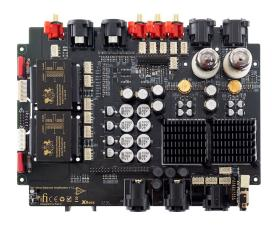
**Left** The bottom level of the multi-layer PCB layout contains the PPCTs – on the left in their shielded enclosures
